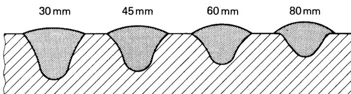
Figure 6. Penetration is reduced as electrical stick-out increases.
