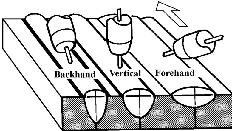
Figure 7. Effect of wire angle on weld penetration and width.
