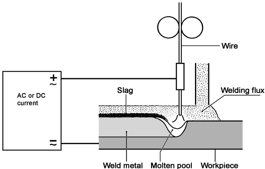
Figure 1. The principle of submerged arc welding.
