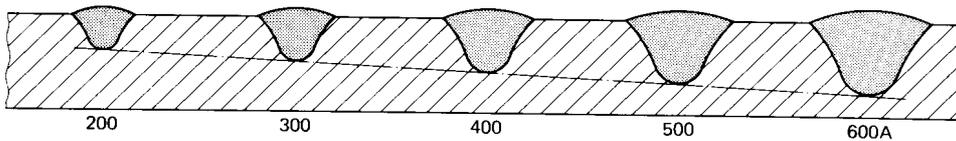
Figure 3. Increasing welding current results in deeper penetration.
